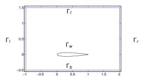
Figure: Flow around an object. Domain including an airfoil.
